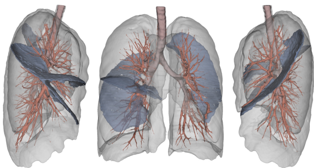
Fig. 3. A sample lung environment showing the segmented anatomy that includes the pleural boundary (gray), major blood vessels (red), airway (tan), and lung fissures that separate lung lobes (blue). These serve as obstacles to the motion planner and create a challenging environment where maximizing reachability will depend on the system design.
