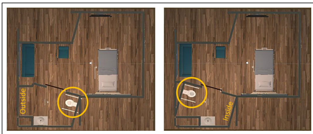
Figure 2. Spatial arrangement of inside (left) and outside (right) toilets. The inside toilet is positioned closer to the bed within the bathroom space, while the outside toilet is further away from the bed. The yellow circles specify the locations of the toilets, highlighting their positions in relation to the surrounding elements. Additionally, the inside and outside walls of the bathroom are tagged.
